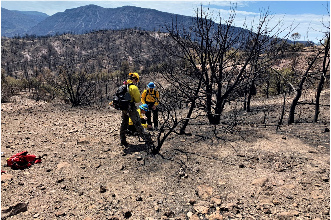
BAER Soil Scientists and Hydrologist Testing Soils in Backbone Burned Area for Water Repellency
